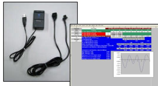
This accessory allows automatic direct entry of measured roller wave data into Excel or other spreadsheet programs using button on digital indicator or on remote cable. Works with RWG-D or RWG-DF gauges. Includes Excel software for easy compliance with new ASTM C1651, "Standard Test Method for Measurement of Roll Wave Optical Distortion in Heat-Treated Flat Glass."
