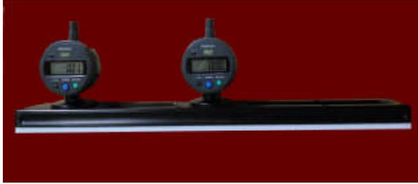
This dual-gauge model has a 16-inch (406 mm) base and is specifically designed for measuring edge-lift (edge curl) in heat-treated flat glass (a requirement of EN 1863-2 and EN12150-2), but can also be used as a flat-bottom roll-wave gauge. Ideal for production control and incoming QC. Controlling edge-lift reduces optical distortion and the chance of field failures in laminated units.
