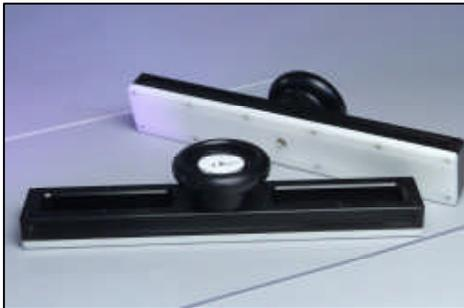
These gauges feature a flat, Delrin-coated bottom surface and dial indicator in inch (RWG-I) or metric (RWG-M) versions. They directly measure peak-to-valley depth ( $W$ ) of the roller wave. The gauge is used with a measuring tape to determine ( $L$ ) the roller wave length (the distance between two consecutive lowest or highest gauge readings).
